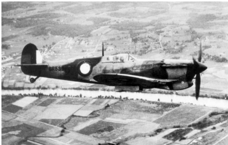
On the 12 th July 1943 Flying Officer Hinds flew Spitfire RAAF Ser A58-45 RAF Ser BR539 DL-X . Pictured here very late 1942 or early 1943 when marked as "X" 54Sqn RAF before DL-X added (Note the Vokes air filter beneath the nose)
